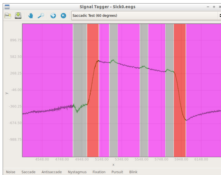
Fig. 2. Signal editor main window. Pink segments mean fixations , gray segments mean noise and red segments mean saccades .
