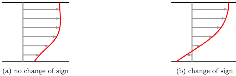
Figure 2: Velocity profile without change of sign (a) and with change of sign (b). We only consider velocity profiles without change of sign in this paper.
