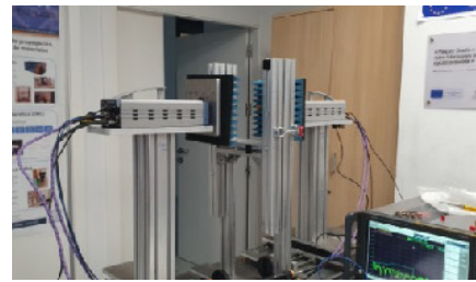
Fig. 1: (a) Measurement scheme used for characterization of materials in free space. (b) Photograph of the setup used for material characterization.
