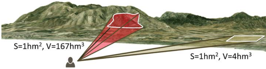
Figure 1 The 3D-perception of an observer located at 6km from two sites: one hilly site and one plain site. The observer sees in both sites the same 2D-viewshed ( 1 \text{ hm}^2 ) but different 3D-viewshed: 167 \text{ hm}^3 in the hilly area and 4 \text{ hm}^3 in the plain area.
