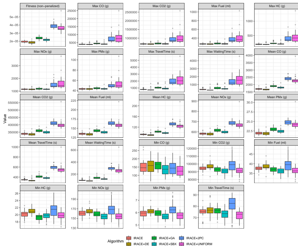
Figure 8: Traffic measures per vehicle. Mean values (and standard deviation) over 30 test traffic scenarios of the median solutions for the algorithms and 1 000 evaluations.
