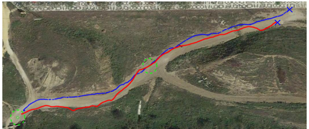
Figure 22. Comparison between reactive and RL paths on the hollow, represented with blue and red lines, respectively.
