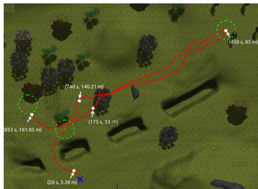
Figure 21. Path followed by the robot with time and distance stamps.
