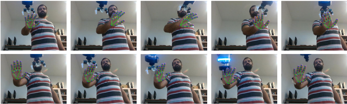
Fig. 5. Consecutive frames (from top to bottom and left to right) of the RGB camera with the MediaPipe solution represented in experiment I. The hand pose changes in different directions and angles whilst the KUKA EE tracks it. Finally, the wristband gets placed around the forearm.
