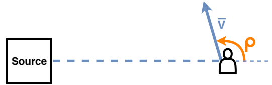
Fig. 3. Angle definition of the Doppler Effect in 2D.
