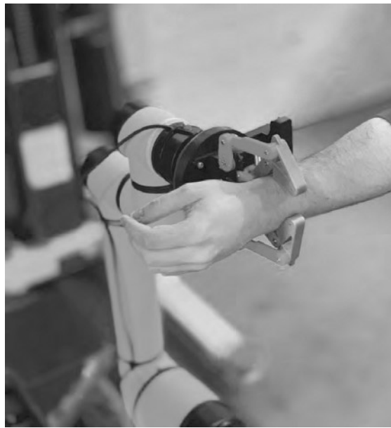
Fig. 1. Manipulator with adaptive gripper for robot-initiated human interaction.
